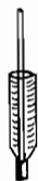
Fig. 4. A modified syringe barrel; a one ml glass syringe barrel which has been shortened to about 2 cm and into which a syringe needle has been inserted and glued using epoxy.
